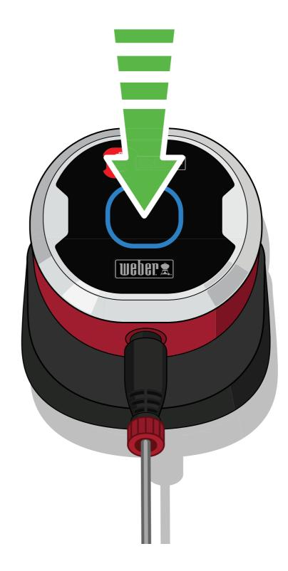
Quickly press and release the power button to turn on the iGRILL MINI. The display will cycle through various colors, then blink blue while waiting to pair.
