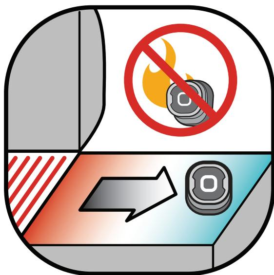
NOTE: The magnetic base is not designed to withstand high heat and it must be placed on a cool surface. If the surface is too hot to touch, it's too hot for the Weber iGrill base!
