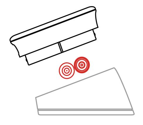
Remove top unit from base, insert batteries
