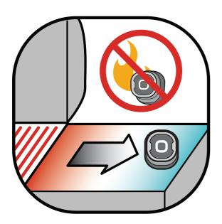
NOTE: The magnetic base is not designed to withstand high heat and it must be placed on a cool surface. If the surface is too hot to touch, it's too hot for the Weber<sup>®</sup> iGrill<sup>®</sup> base!
